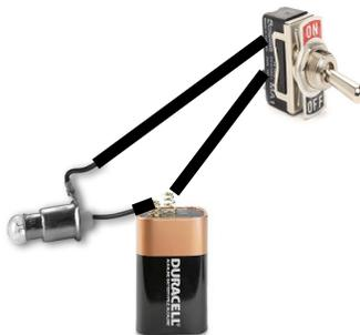
The bulb goes bright or dark in direct sympathy with the switch going on or off. The difference between this switch and an isolated one is that we surrounded this one with circuitry (wires, bulb) so it became part of a larger whole.
